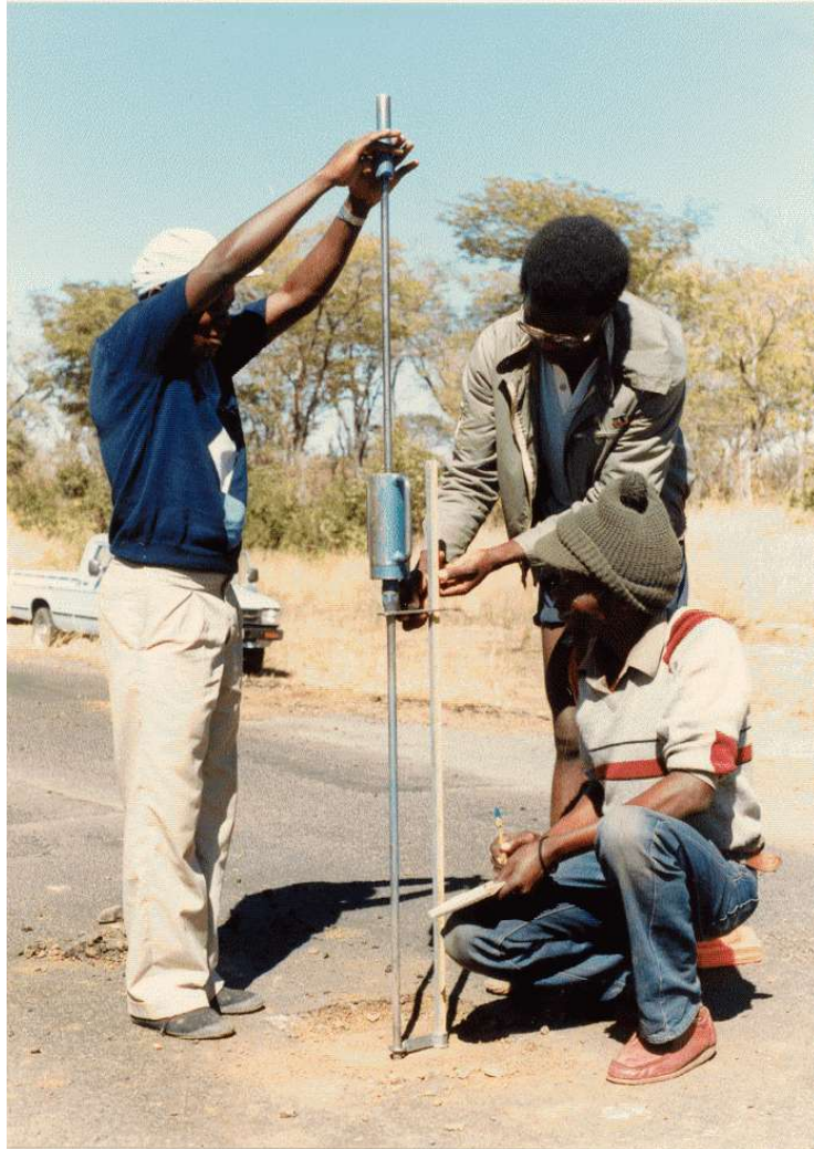
DCP test in process
